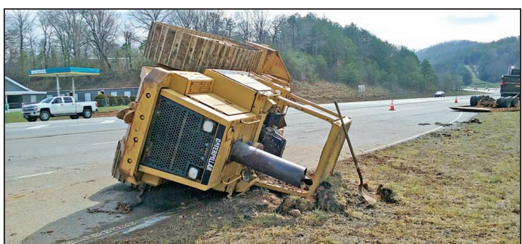
A ratchet binder snapped during GDOT's transportation of this medium-sized bulldozer last week, causing it to turn over onto the side of Georgia 515
