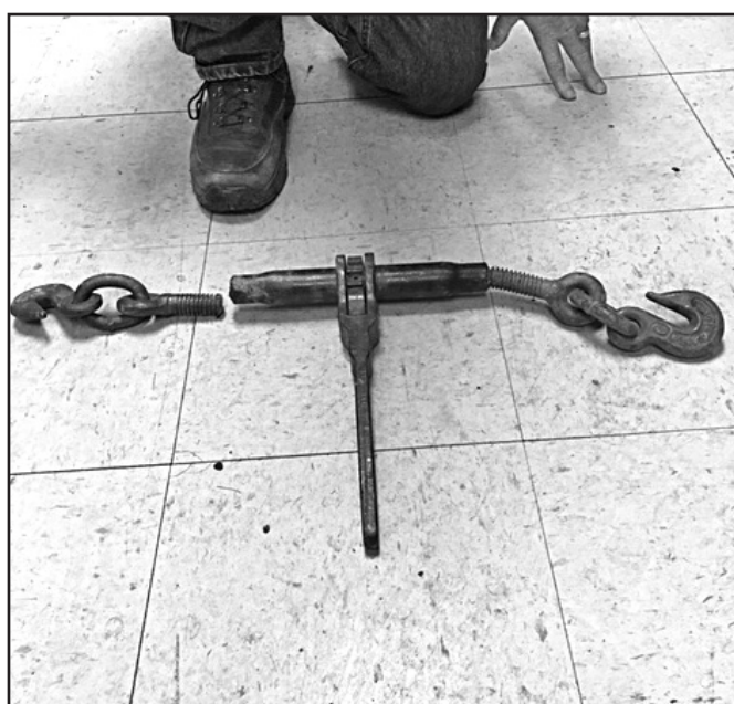
Broken ratchet binder.
